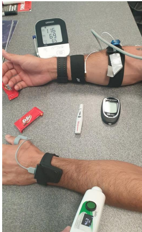
Figure 2: Sensors worn for the first 2 trials of the UofM dataset collection procedure
