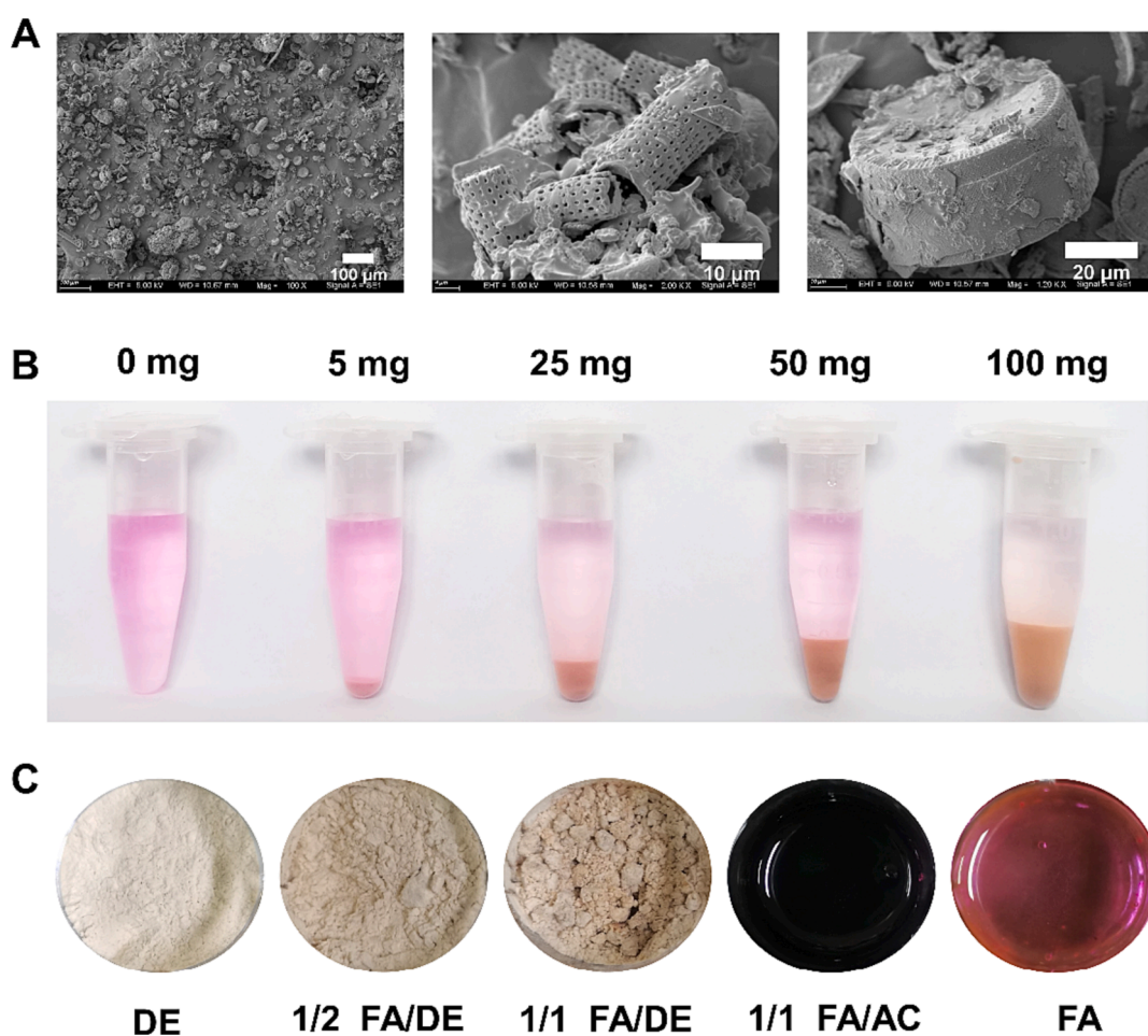
Fig. 5. The adsorption properties of DE (A) SEM image of DE. (B) Adsorption capability of small molecular dye by DE. Adsorption of Rhodamine B (RhB) by different amount of DE in aqueous solution. (C) Oil adsorption test of DE. The DE or activated carbon (AC) adsorption of Rhodamine B (RhB) containing fatty acids (FA) with different weight ratios.
